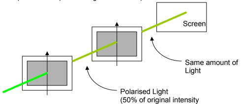
If the directions of both polarisers are at right angles to each other (called crossed polarisers), then no light will pass through.
