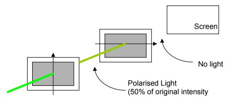
For other angles, the amount of light getting through to the screen vary from almost all if the second polariser is nearly aligned, to next to nothing if the polarisers are almost crossed according to Malus' Law.
