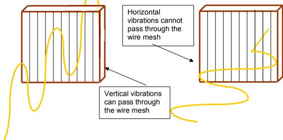
In a similar way, optical devices called polarisers only allow light with a specific polarisation to pass through them. This is commonly called plane polarisation.
