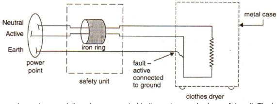
The figure above shows a clothes dryer connected to the mains supply via a safety unit. The iron ring is an essential part of the safety unit. The active and neutral wires run through the ring. The clothes dryer has an electrical fault, a connection between the active wire and the earthed metal case of the dryer.
