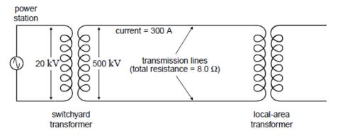
The RMS current in the secondary of the switchyard transformer is 300 A. Assume the two transformers are ideal.
