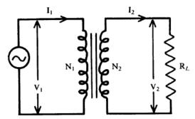
Assume that power transfer through the transformer is 100 per cent efficient.
