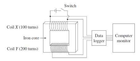
A student closes the switch for a short time, then opens it. The data logger records values of voltage for both coils for the duration of the investigation. The data logger software displays the results as a pair of voltage–time graphs on a computer monitor.
