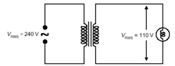
There are 1440 turns on the primary coil of the transformer.
