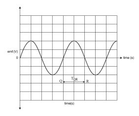
Since the loop is rotated at a rate of 10 revolutions per second, it must take 0.1 secs for each revolution.
