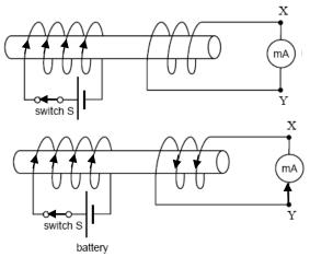
This will create a North pole at the left hand end of the iron core. To oppose this, the induced current will create a North pole at the extreme right hand end of the iron core. This will lead to a current as shown below. Therefore the momentarily induced current will be from Y to X.
