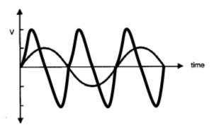
The new graph should have double the amplitude and half the period.
