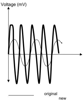
The graph remains a sine curve, but the  $\underline{\textit{amplitude doubles}}$  , the induced EMF is given by
