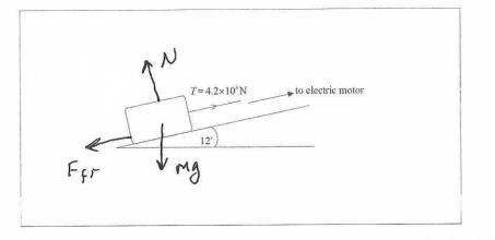
20. A stone block is pulled at constant speed up an incline by a cable attached to an electric motor.
