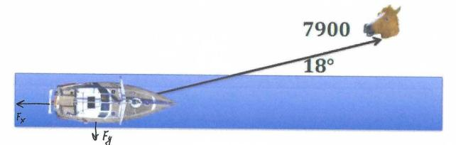
The mass of the barge is 9500 kg and the magnitude of its acceleration is 0.12 m/s<sup>2</sup>. Calculate the drag force exerted by the water on the barge. (Do not include the buoyancy force as this is not a drag force.) Give both magnitude and the direction. Hint: the drag force from the water does not point in the same direction as the rope! Show your working. (9 marks)
