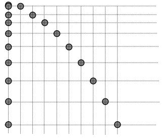
The interval between the lines represents how far the ball has travelled in a small time interval. Notice that the distance between the horizontal lines increases as the ball descends, indicating that the ball is speeding up. The distance between successive vertical lines remains constant, indicating that the ball is travelling with a constant velocity in the horizontal direction.
