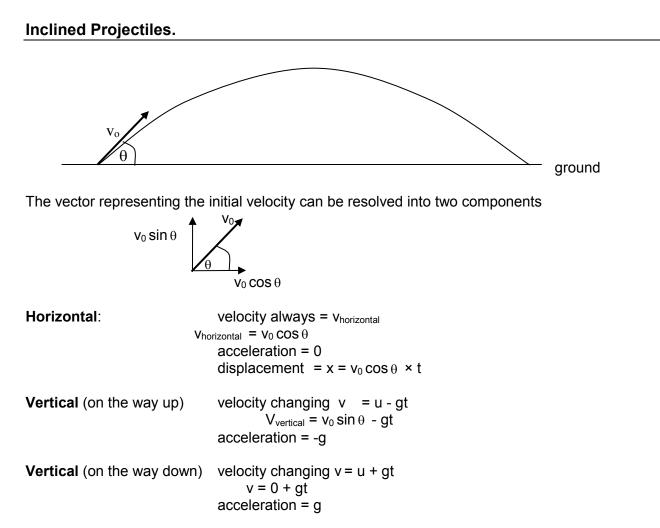
The displacement at any time of the motion is:  $y = ut - \frac{1}{2} gt^2$  (The same on the way up and down).
