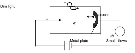
The experiment can be used to show that the number of electrons ejected depends upon the light intensity. As the light intensity increased, so too did the size of the current. More electrons were escaping from the metal when the light was brighter.
