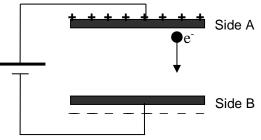
If an electron is fired through a gap into a region between two plates, then the electric field will oppose its motion. If the electron is travelling relatively slowly, the field may stop the electron before it reaches the other side. The electron will then travel in the opposite direction. If the electron is going fast enough (i.e. has sufficient initial kinetic energy, then it may reach the plate before it slows to a stop.
