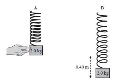
Figure A shows an ideal spring with a 2.0 kg mass attached. The spring-mass system is held so that the spring is not extended. The mass is **gently** lowered and the spring stretches until, in Figure B, the spring-mass system is at rest. The spring has extended by 0.40 m.
