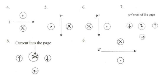
5. Using arrows, X's or dots, indicate the requested variable for each questions using the right hand rules.
