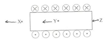
19. Cross-section of the solenoid with the current shown. Indicate which end of the solenoid becomes the north pole and which south. Explain why solenoid becomes an electromagnet. Draw2 lines of magnetic field.
