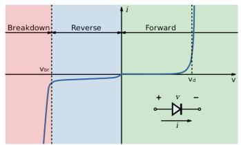
LEDs use a p-n junction to create these specific conditions. This is where a p-type semiconductor (which contains free positively charged carriers, known as holes) and an n-type semiconductor (which contains free negatively charged carriers, electrons) join. These junctions are the building blocks of every semiconductor electronic device.
