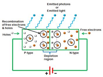
in the valence band they release energy in the form of photons. This phenomenon is called electroluminescence, the emission of light from a semiconductor under an electric field. Luminescence is different to other kinds of light emission, such as incandescence, because it provides no heat. Other kinds of luminescence include chemiluminescence (as in glow sticks) and phosphorescence (glow in the dark paint).
