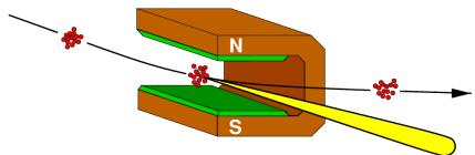
The radiation that comes off a synchrotron can be manipulated by how tight the bend is, and this radiation can be very useful for different purposes. The radiation comes off a synchrotron at a tangent to the circle.
