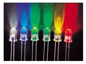
Light Emitting Diodes **(LED's)** are diodes that emit light when a current passes through them at a suitable voltage. Their V-I graphs are similar to that of an ordinary diode.
