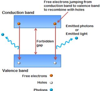
All diodes emit photons but not all diodes emit in the visible spectrum. The material in an LED is selected based on the desired emission
