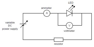
With the blue LED in the circuit the supply voltage is gradually increased. The LED does not emit light until the voltage reading on the voltmeter is 2.64 V. At this time there is a current of 5.00 mA read on the ammeter, A.
