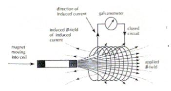
As the north of the magnet is pushed toward the solenoid, an EMF is induced that will oppose this movement. The left end of the solenoid will act as a North Pole to repel the magnet.
