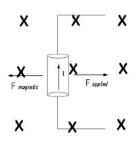
In the diagram, the wire is being moved to the right due to an applied force  ${\bf F}_{\rm applied}.$
