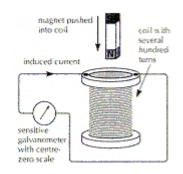
Note: An emf ( $\xi$ ) and hence a current, are induced in the solenoid when the magnet is moving into, or out of, the solenoid. The size of the emf ( $\xi$ ) depends on the speed of movement and the number of turns on the solenoid, as well as the strength of the magnet.
