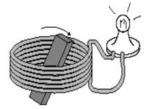
The creation of an electric current in a conductor by changing the magnetic <u>flux</u> is called Electromagnetic Induction. The effect was discovered by the British physicist Michael Faraday and led directly to the development of the rotary electric generator, which converts mechanical motion into electric energy.
