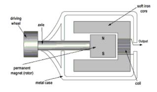
When a simple electric motor is set up so that the magnetic field is present, but the coil is not connected to a source of emf, a current can be generated in the coil by rotating it mechanically.
