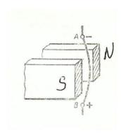
5. This question relates to the picture in question 4. If strength of magnetic field is 10 mT, current in the wire is 3 A and length of wire in magnetic field is 15 cm, calculate the size of the force acting on the wire.
