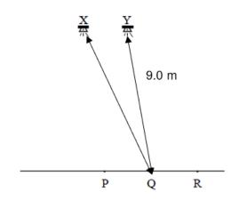
The point Q is the first nodal point from the central maximum at P. So the path difference between XQ and YQ must 0.5  $\lambda$ .
