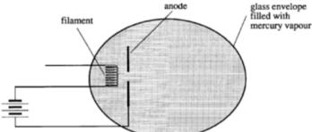
Inside a sealed glass vessel filled with mercury vapour, electrons are accelerated from a hot cathode by a potential difference of +8.0 volt applied between the filament and the anode. They pass through a hole in the anode and thence through mercury vapour. The student examines the spectrum of radiation from mercury atoms in the path of the electrons.
