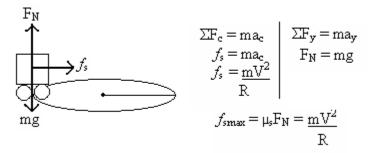
In this case friction force is the net force, so centripetal force equal friction force and perpendicular to the velocity. If  $F_{fr\ max} < \frac{mv^2}{r}$  object will slide away from the centre until increase in radius will make them equal again (remember this when you will be driving the car!).
