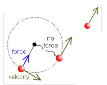
The formula for the magnitude of a net force necessary to keep an object in circular motion (such force is called centripetal force. Centripetal force is a <u>net</u> force. There is no such separate  $u^2$
