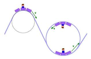
To solve those problems we should write resolution of the second Newton's law into the vertical direction.
