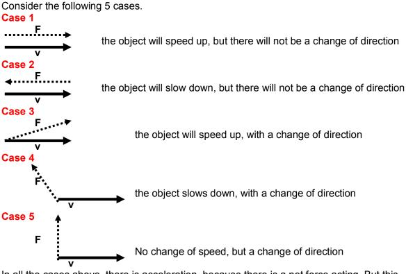
In all the cases above, there is acceleration, because there is a net force acting. But this acceleration does not always result in a change of speed. Remember that velocity is a vector, and has a magnitude *and* a direction.
