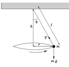
In this case net force (centripetal force)  $F_c = T \sin \theta$  (resolution of the second Newton's law in the horisontal direction) and  $T \cos \theta - mg = 0$  (resolution of the second Newton's law in the vertical direction).  $F_c = \frac{mv^2}{r}$
