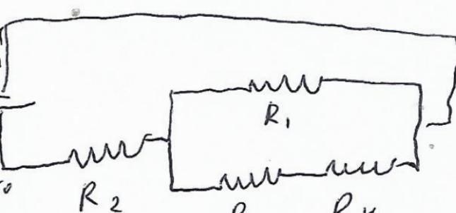
$$V_{R_1} = 11 - 6.3 = 4.7 \text{ V} \quad I_{R_1} = \frac{4.7}{1000} = 4.7 \mu\text{A}$$
