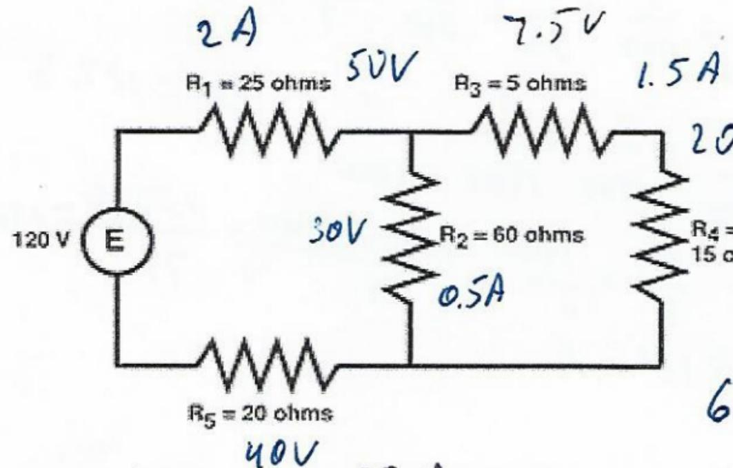
$$V_{R_3} = 2 \times 20 = 40V$$
