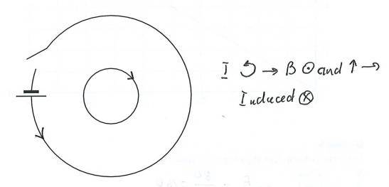
Which one of the following best describes the induced current in the inner loop once the switch is closed in the outer loop, as viewed from above?
